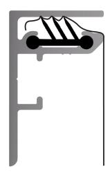
EASITEX has an internal "grip-strip" which clamps the fabric firmly into position leaving you with a great and hassle-free finish.
